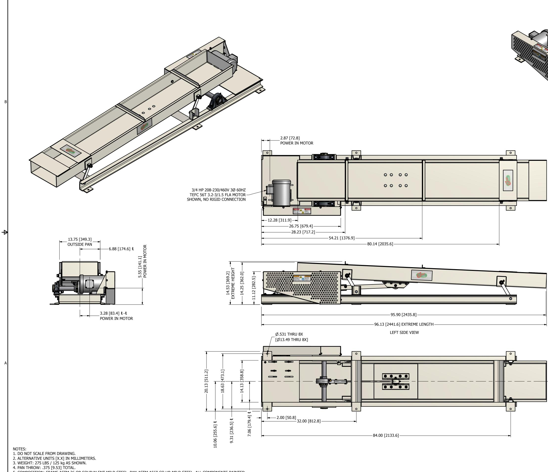
5. COMPOSITION; FRAME ASTM 36 OR EQUIVALENT MILD STEEL, PAN ASTM A569 CQ HR MILD STEEL. ALL COMPONENTS PAINTED.
