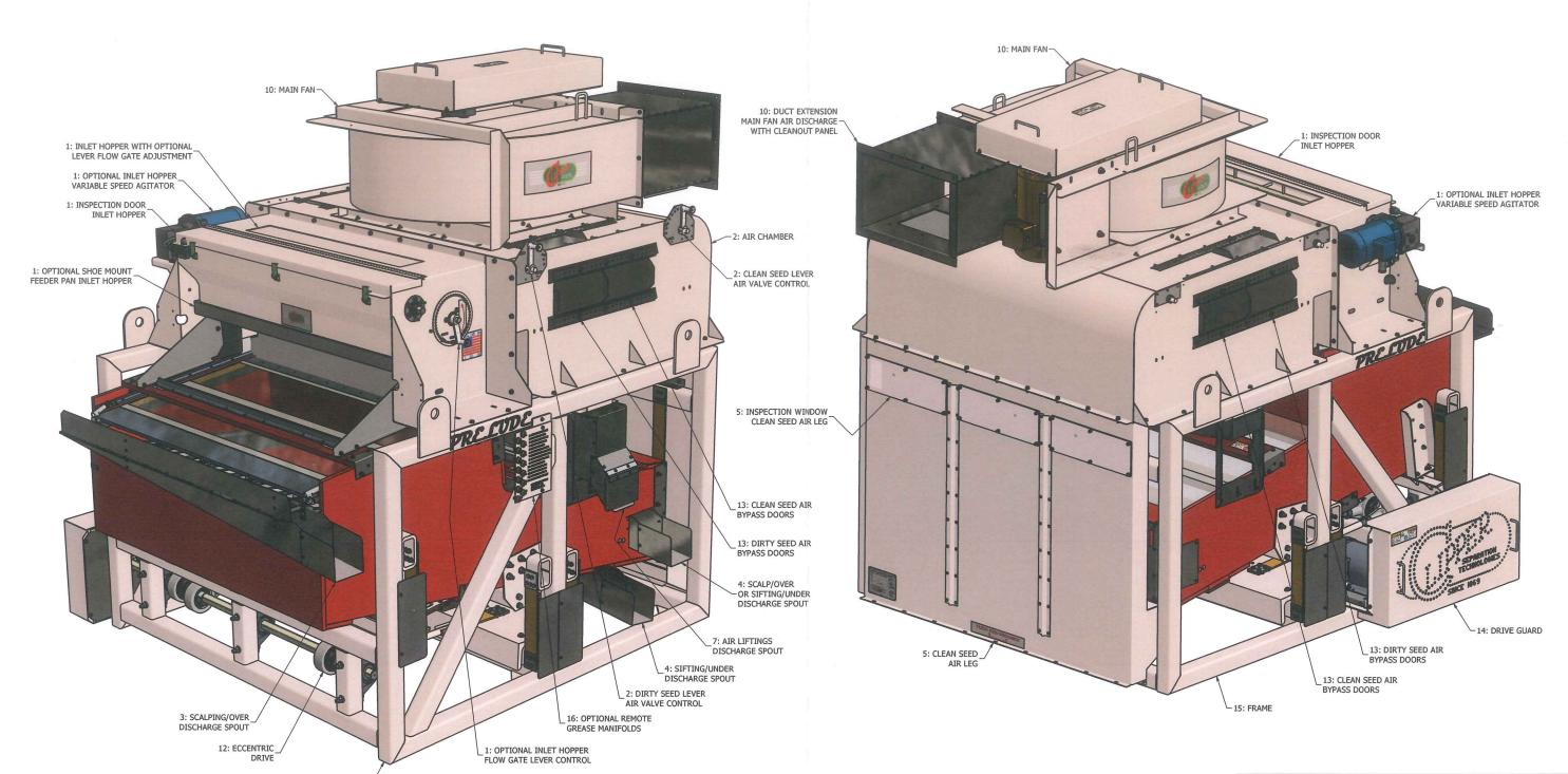
GENERAL DIMENSIONS: EXTREME HEIGHT: 91.5" [2324 mm]. EXTREME WIDTH: 85.5" [2172 mm]. EXTREME LENGTH: 100" [2540 mm]. FLOOR WIDTH: 69.5" [1765 mm]. FLOOR LENGTH: 73.4" [1864 mm].
