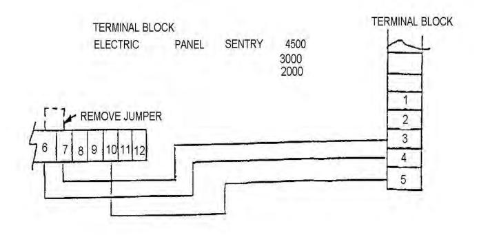
Jumper must be installed between 15 amp Fuses load side line 1 and terminal 9 In mill panel.
